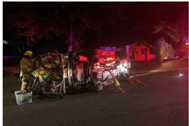
Rollover Accident with Stabilization
