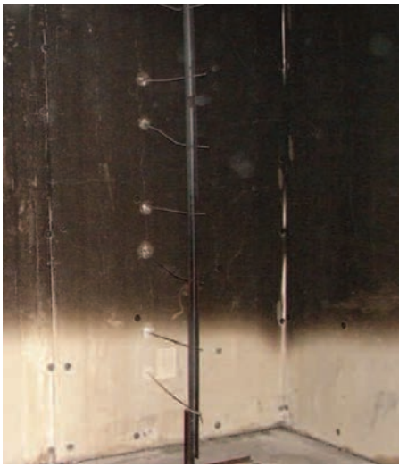
Figure C-9: Burn Room Thermocouple Array Figure C-10: Target Room Instrument Cluster
