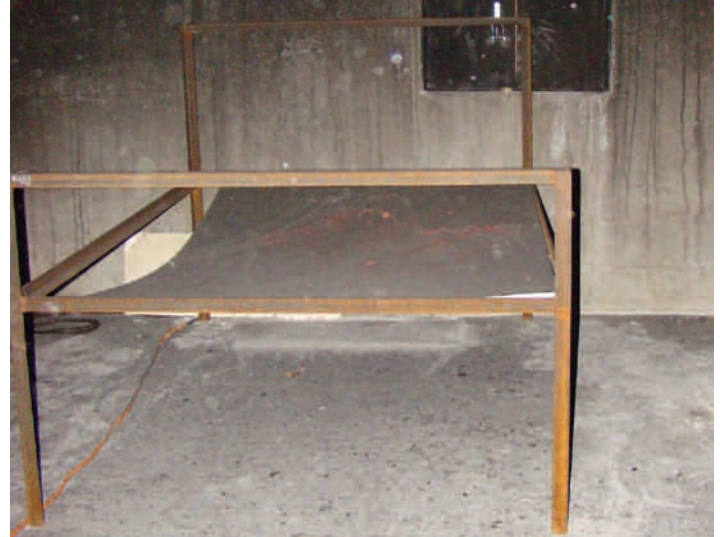
Figure 5: Noncombustible Furniture Used in the Time-to-Task Experiments
