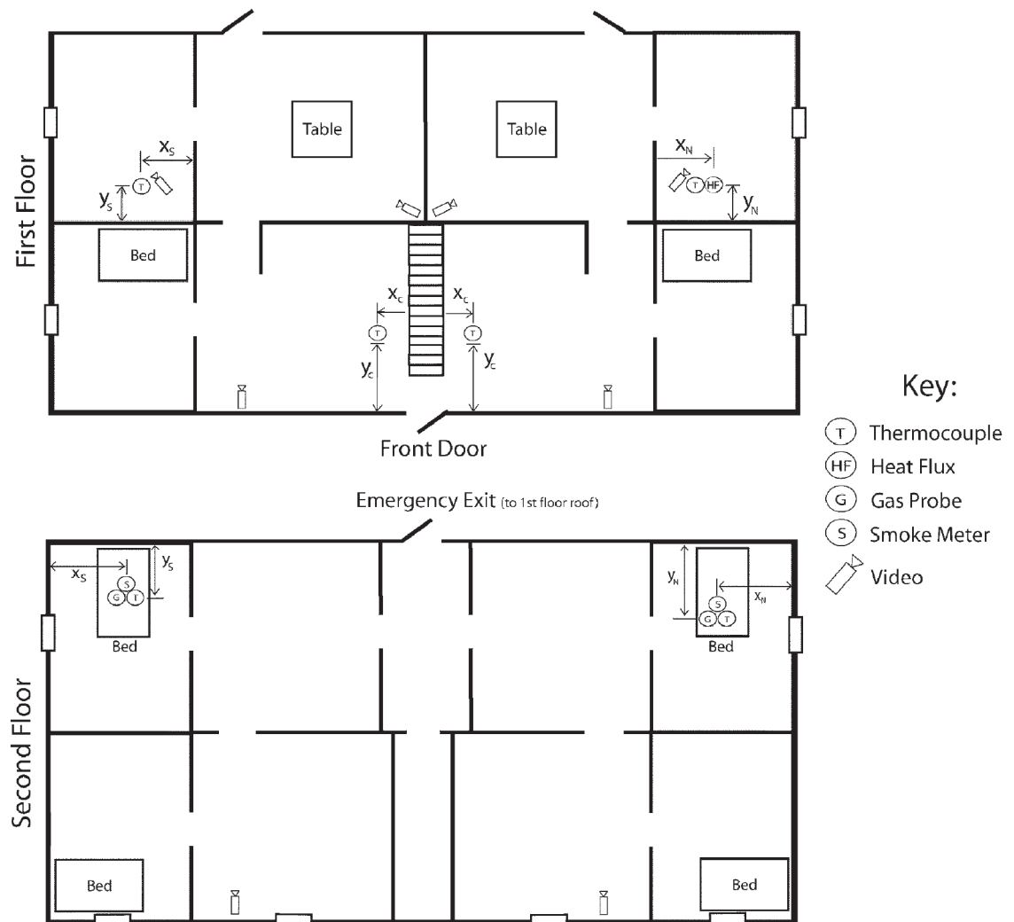
Figure 6: Instrumentation and Furniture Prop Layout
