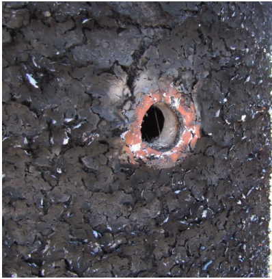
In fire-testing at the Southwest Research Institute, the entire length of Shakespeare poles were protected and little-to-no charring was observed on interior structural glass. After a fire, remediation procedures are available for charred products.
